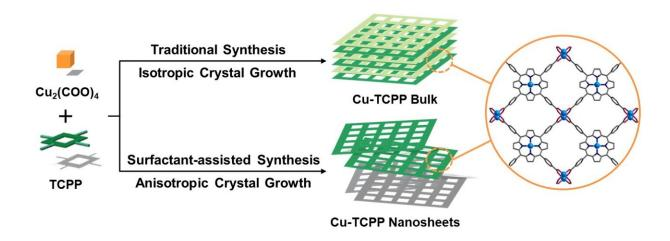
The preparation of MOF nanosheets via traditional vs. surfactant-assisted methods. Credit: NIMTE
