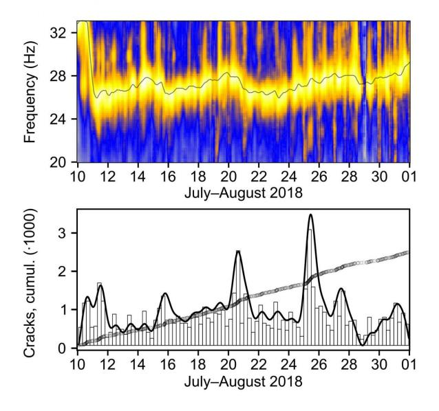
The researchers observe a characteristic sawtooth pattern in the frequency of the mountain (top): it rises with the stress in the rock and drops again after days. In the process, seismic signals are registered (bottom), which occur when rock cracks open. If the cycles become shorter, a mass break-up is approaching. This is also a danger indicator. Credit: Dietze/GFZ
