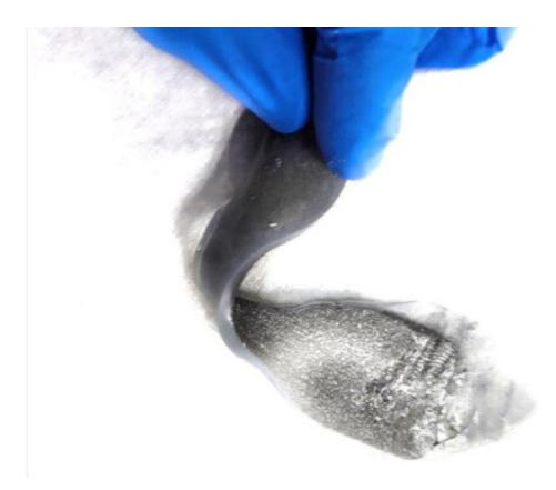
Liquid metal composites enable soft, stretchable circuits that are electrically conductive, mechanically self-healing, and highly adaptable. Credit: Soft Machines Lab, Carnegie Mellon University
