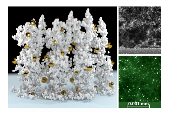
Main pic: Artist's impression of the 3-D nanoparticle scaffold, consisting of metallic nanoparticles (yellow) embedded within semiconductor nanoparticles. Credit: The Australian National University
