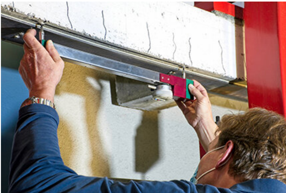
Measuring the change in length at the bottom of the beam. Credit: Empa
