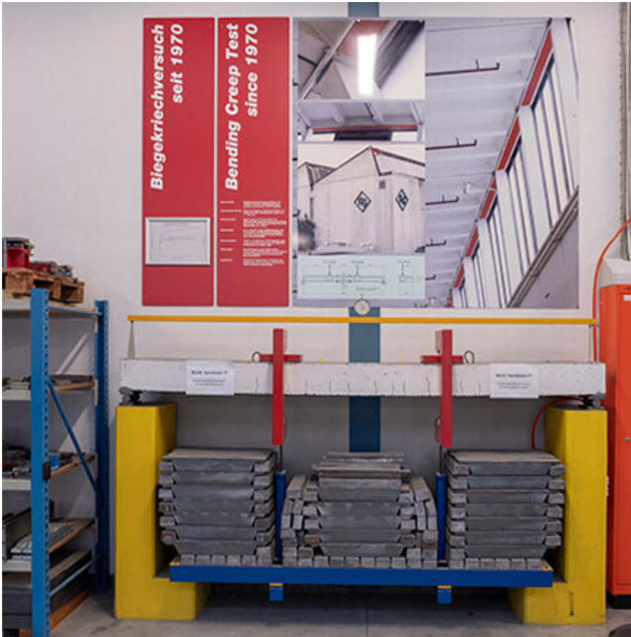
The concrete beam strengthened with a steel plate—"glued"—has carried a load of just over six tonnes since 24 March 1970. Credit: Empa
