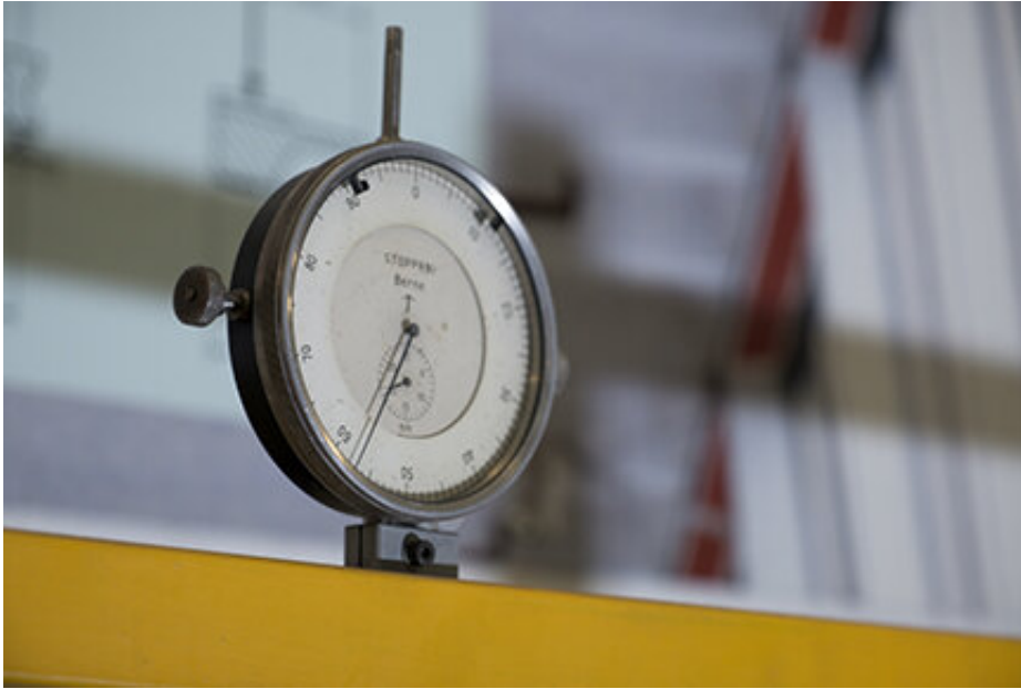
Instrument for measuring deflection. Credit: Empa
