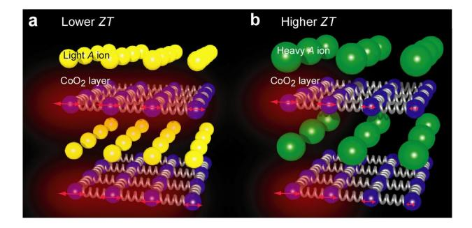
Hypothesis for the ZT improvement of layered cobalt oxide. Ions with greater atomic mass (right) would increase ZT as they suppress thermal conductivity in the cobalt oxide layers. Credit: Yugo Takashima et al, *Journal of Materials Chemistry A*, October 13, 2020
