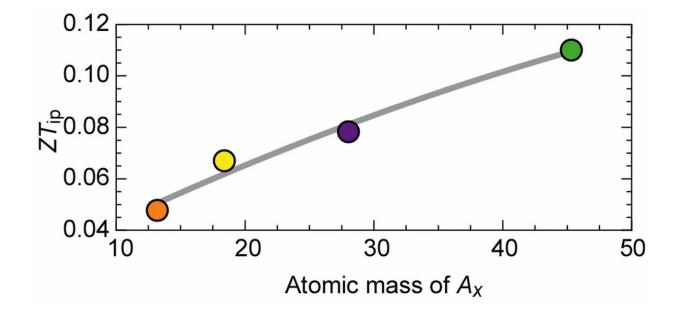
Correlation between the atomic mass and thermoelectric figure of merit (ZT). As the atomic mass of the alkali or alkaline earth metal increases, the ZT also increases. Orange, calcium; yellow, sodium; purple, strontium; green, barium. Credit: Yugo Takashima et al, *Journal of Materials Chemistry A*, October 13, 2020
