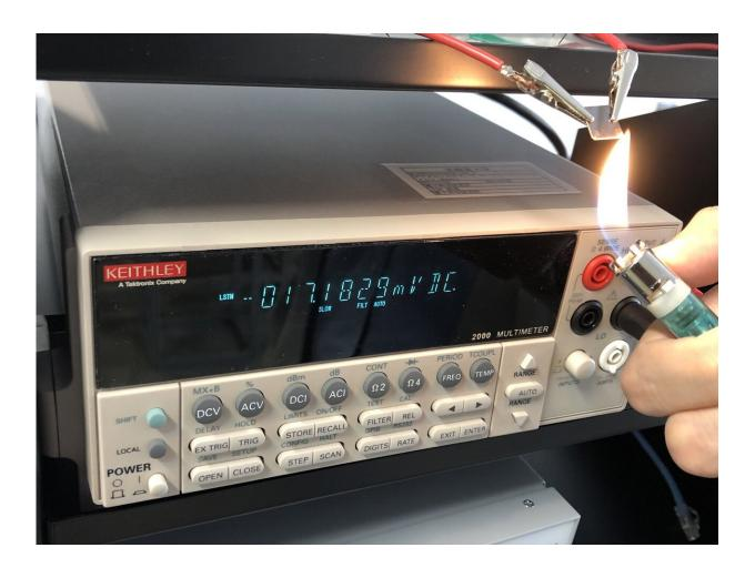
The barium-cobalt oxide film (top right, approximately 1 cm2) being exposed to an open flame to generate voltage. Credit: Hiromichi Ohta
