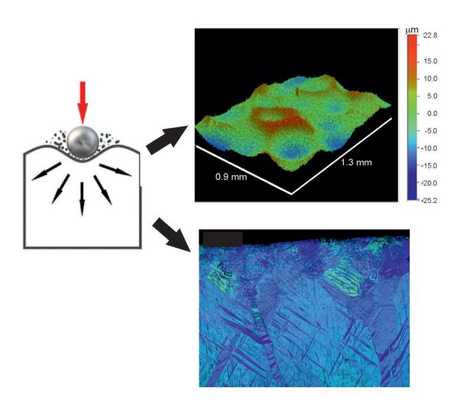
Surface mechanical attrition treatment (SMAT) of magnesium improves its strength and corrosion resistance. Credit: IFJ PAN
