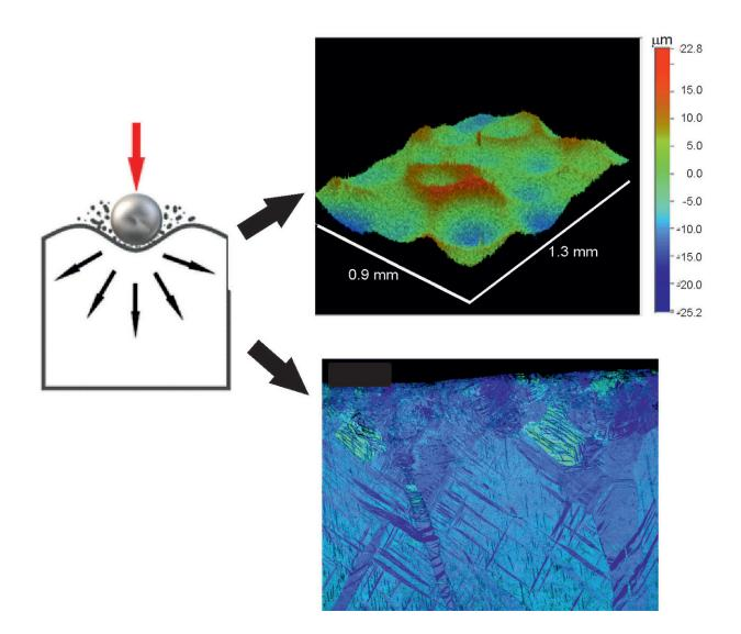
Surface mechanical attrition treatment (SMAT) of magnesium improves its strength and corrosion resistance. Credit: IFJ PAN
