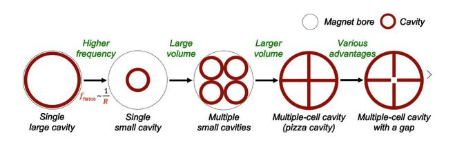
Figure 1. Cavity designs with various internal sections. (Left to right) (1) single large cavity, (2) single small cavity, (3) multiple small cavities (4) multiple-cell cavity (pizza cavity) (5) multiple-cell cavity with a gap . Credit: IBS
