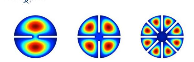
Figure 2. Cross-sectional view of various multiple-cell (double-, quadruple- and octuple-cell) cavities with the expected distribution of the axion-induced electric field (from simulation). Credit: IBS
