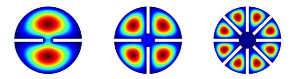
Figure showing the cross-sectional view of various multiple-cell (double-, quadruple-, and octuple-cell) cavities with the expected distribution of the axion-induced electric field by the resonant mode of interest. Credit: Jeong et al.
