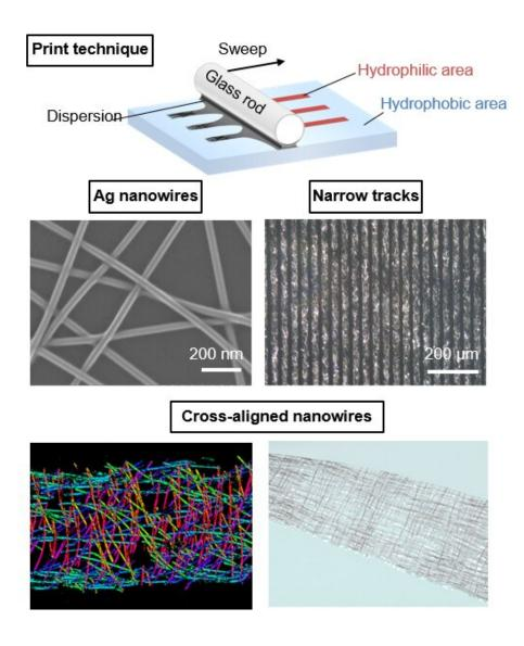
Wet-process of Ag nanowires-based transparent electrode and cross-aligned nanowires. Reprinted with permission from our achievement in *Advanced Intelligent Systems*. Credit: *Advanced Intelligent Systems*
