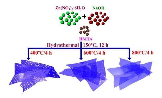
ZnO nanosheets were thermally treated at three different temperatures (400, 600, & 800°C) to tune their hole density. The hole density consistently reduced as the temperature was increased from 400°C to 800°C. Credit: Manjeet Kumar, Incheon National University
