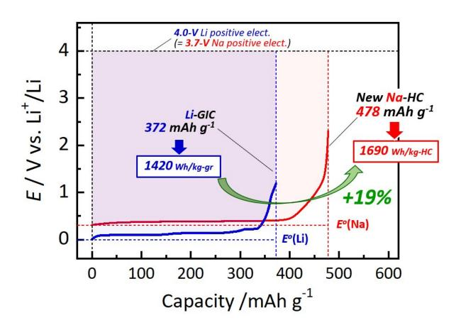
The higher capacity of this new hard carbon electrode material means that a 19% increase in energy density by weight is possible in sodium-ion batteries compared with lithium-ion batteries Credit: Shinichi Komaba from Tokyo University of Science
