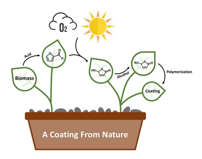
Lignocellulose biomass is cracked using acid to produce furfural. Using visible light and oxygen, furfural is converted into hydroxybutenolide, which is then modified using different alcohols to produce alkoxybutenolide monomers, that can be polymerized into coatings using UV light. Credit: George Hermens and Paco Visser, University of Groningen
