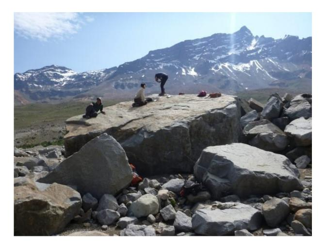
Team members remove bits from a boulder left behind by a shrinking glacier. Back in the lab at Lamont, they can measure the levels of beryllium-10 in the sample in order to determine how long ago it was deposited. Credit: Mike Kaplan
