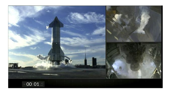
This frame grab from video posted on the SpaceX Twitter page shows views of SpaceX's futuristic Starship just after an automatic engine abort occurred with just 1.3 seconds remaining in the countdown to liftoff of its first high-altitude test flight, Tuesday, Dec. 8, 2020, in southeast Texas. (SpaceX via AP)
