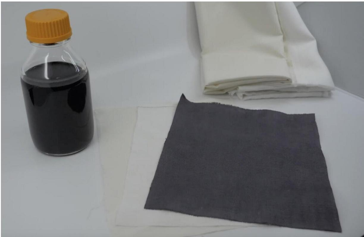
Coating standard cotton or linen fabric with a solution of MXene material can imbue it with substantial electromagnetic shielding capabilities, according to new research from Drexel University. Credit: Drexel University
