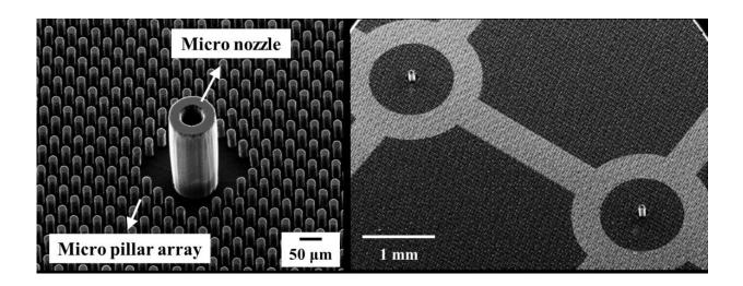
Figure 1. Polymer micro-nozzle array. Credit: The Korea Advanced Institute of Science and Technology (KAIST)
