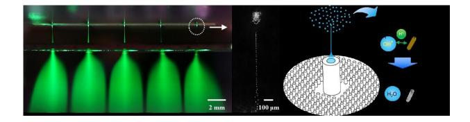
Figure 2. The multiplexed electrospray of water and antimicrobial effect. Credit: The Korea Advanced Institute of Science and Technology (KAIST)
