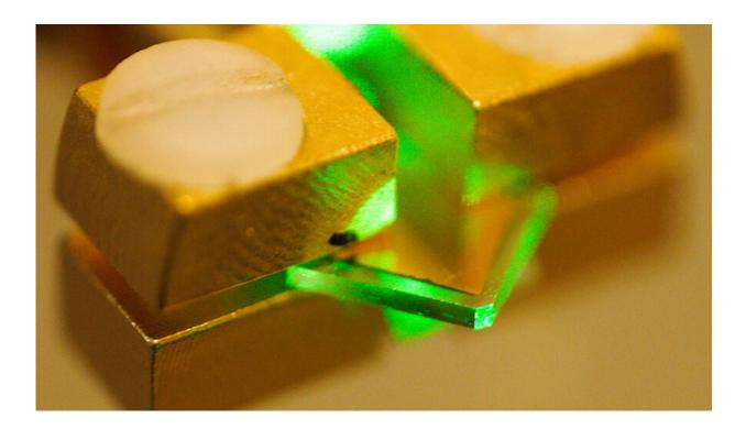
A photoconductive switch made from a synthetic, chemical vapor deposition diamond under test. Credit: Lawrence Livermore National Laboratory
