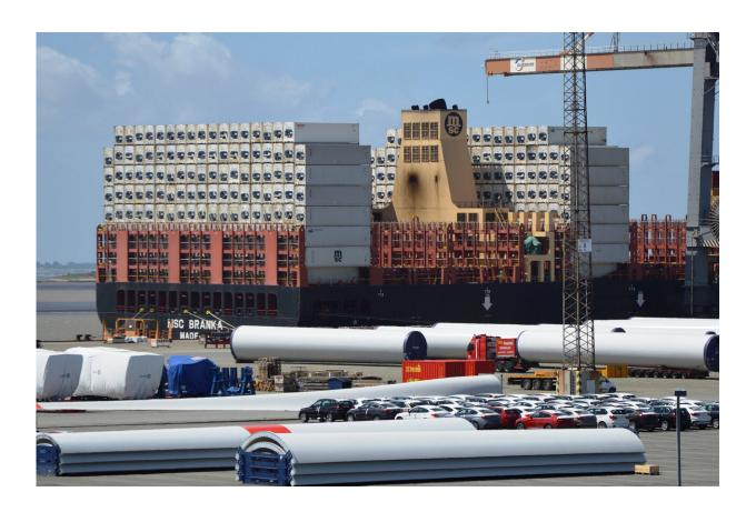
The growing demand for cooling technologies is accompanied by steadily increasing energy requirements. In addition, conventional cooling systems rely on refrigerants with a very high global warming potential. The image shows integral reefer containers stacked on a container ship. Credit: Wikimedia commons, Licence: CCO 1.0
