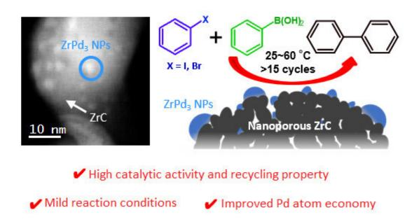
Overview of the novel Pd–ZrC heterogeneous catalyst. The new catalyst consists of ZrPd3 nanoparticles grown on an inert ZrC support. Its simple fabrication procedure, coupled with its many advantages over available alternatives, make the proposed catalyst an attractive option for Suzuki cross-coupling reactions. Credit: Tokyo Institute of Technology
