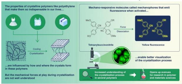
Crystallization-induced Mechanofluorescence for Visualization of Polymer Crystallization
