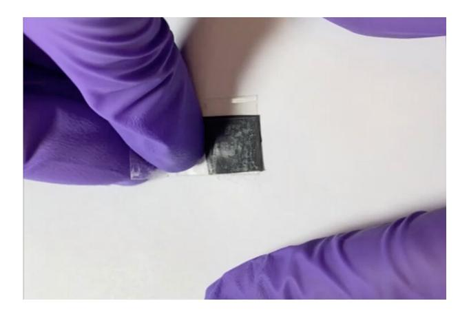
Water-based latex paint sticks so tightly to the oxidized polyethylene, referred to as Ox-LDPE, that Katerina Malollari was unable to remove it with tape, even after 11 attempts. Latex does not adhere to normal plastics. Credit: UC Berkeley photo by Katerina Malollari
