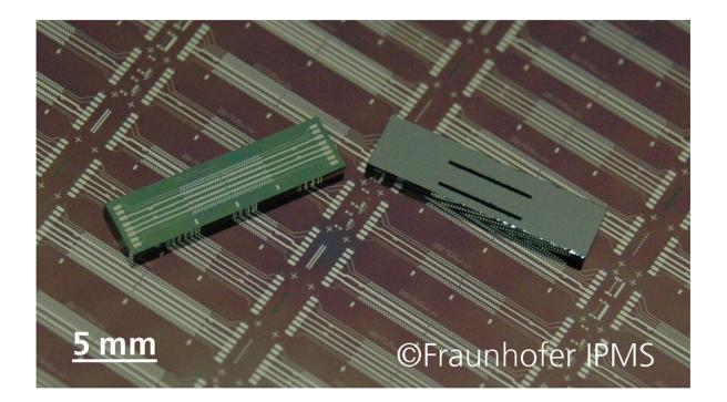
At the heart of this novel ion-mobility spectrometer is a miniaturized FAIMS chip. Credit: Fraunhofer IPMS
