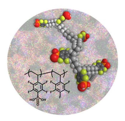
Researchers have developed a proton conductor for fuel cells based on polystyrene phosphonic acids that maintain high protonic conductivity at high temperatures without water. Credit: Los Alamos National Laboratory
