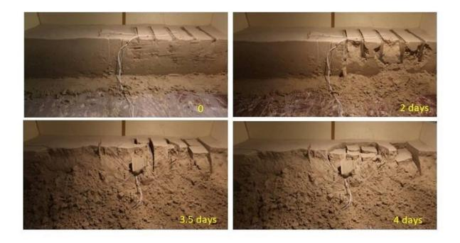
Simulated thawing of 2.5-m-wide block of permafrost, in cold room. In each photo, the left half of the block models a homogeneous frozen soil with low ice content, and the right half models an ice-rich permafrost with vertical ice wedges. The experiment demonstrated that ice-rich permafrost undergoes extensive erosion while thawing. Credit: F. Costard, GRL/AGU 2020, Article ID: GRL\_61641
