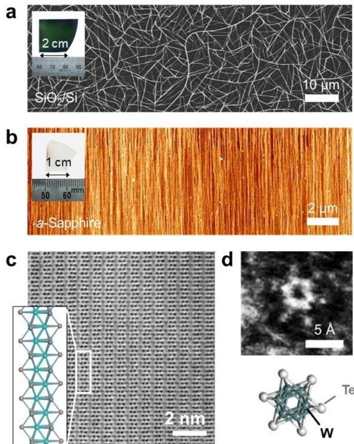
(a) Scanning electron microscopy picture of nanowires grown on a silicon/silica wafer. (b) Atomic force microscopy image of nanowires grown on a crystalline
