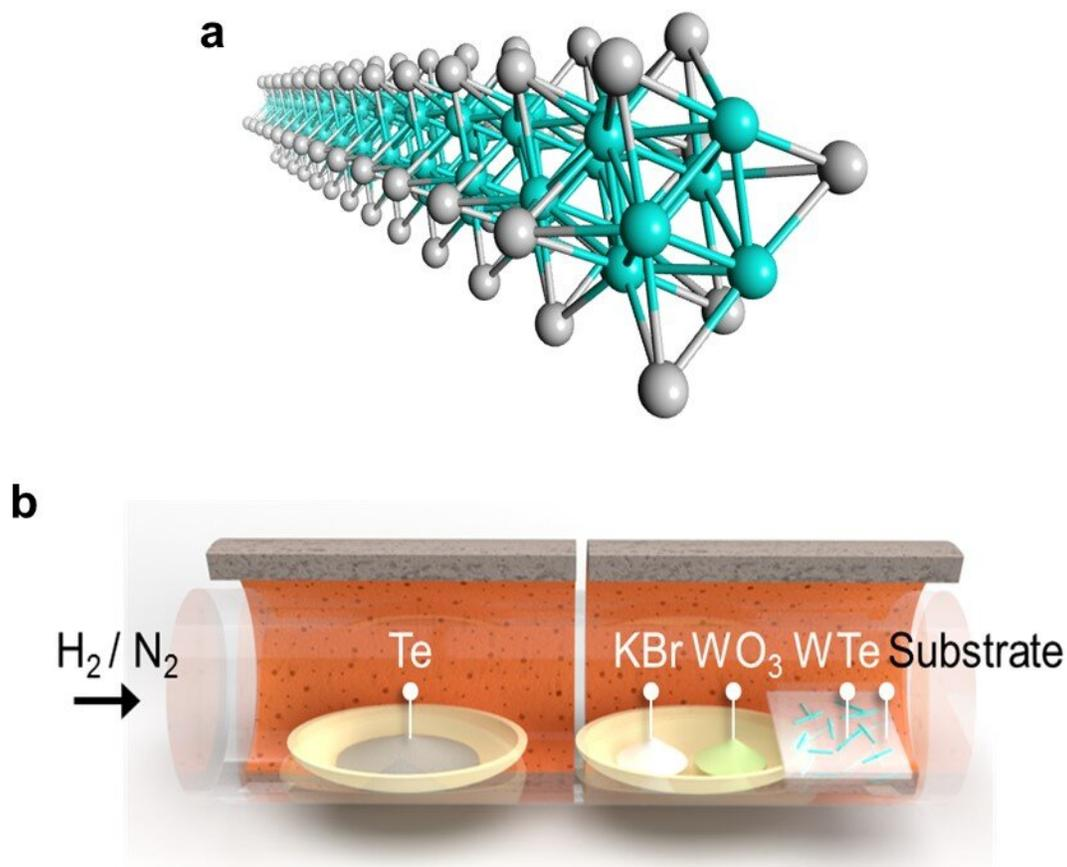
(a) Illustration of a TMC nanowire (b) Chemical vapor deposition. The ingredients are vaporized in a hydrogen/nitrogen atmosphere and allowed to deposit and self-assemble on a substrate. Reprinted with permission from Ref. 1
