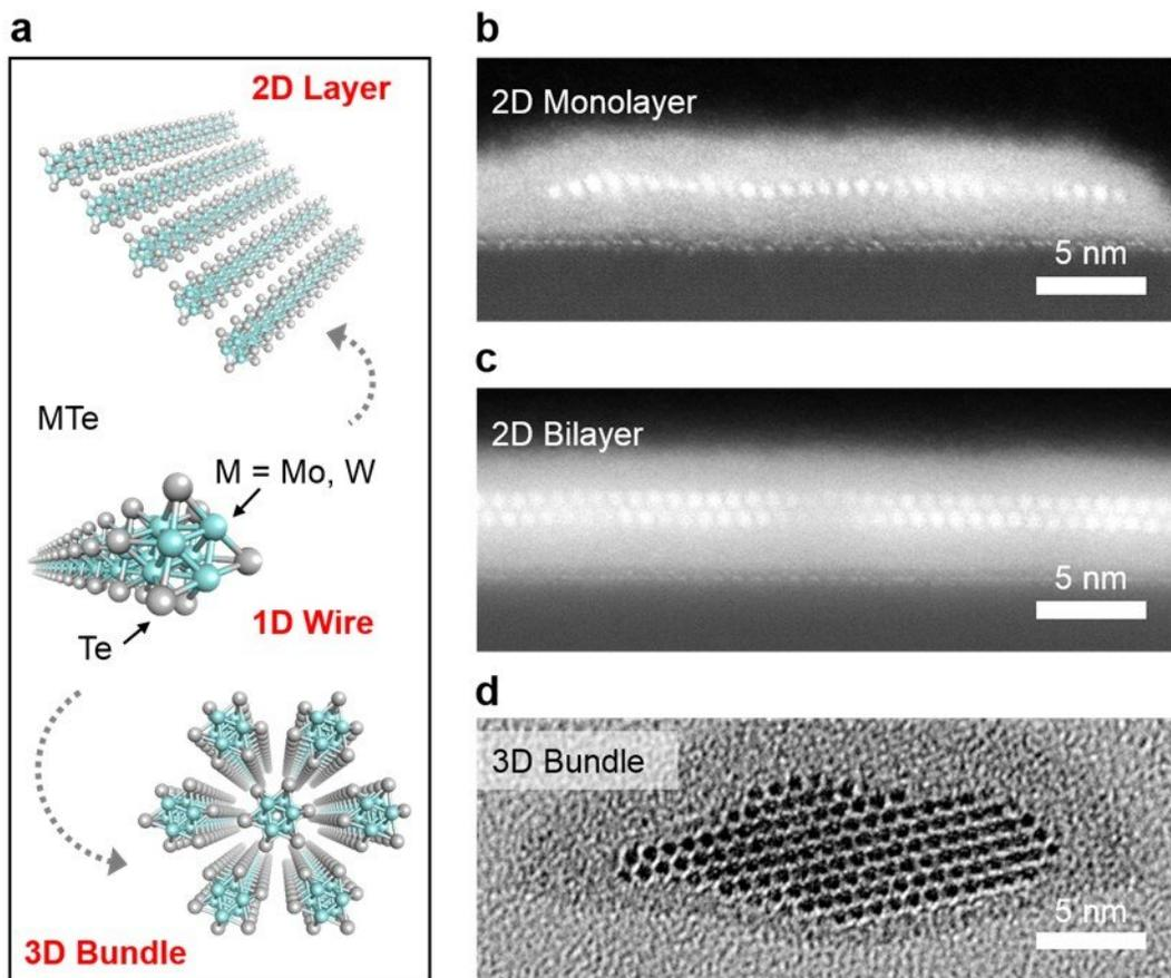
(left) (a) Illustration of different forms of TMC assembled on the substrates. Scanning transmission electron microscopy images of the cross-section of (b) a monolayer of nanowires, (c) a bilayer of nanowires, and (d) transmission electron microscopy image of 3D bundles. Reprinted with permission from Ref. 1 Credit: American Chemical Society (ACS)
