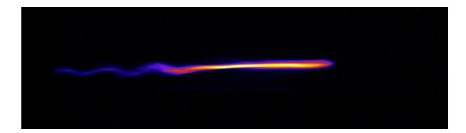
Electrons are ejected from the plasma accelerator at almost the speed of light, before being passed through a magnetic field which separates the particles by their energy. They are then fired at a fluorescent screen, shown here. Credit: Rob Shalloo
