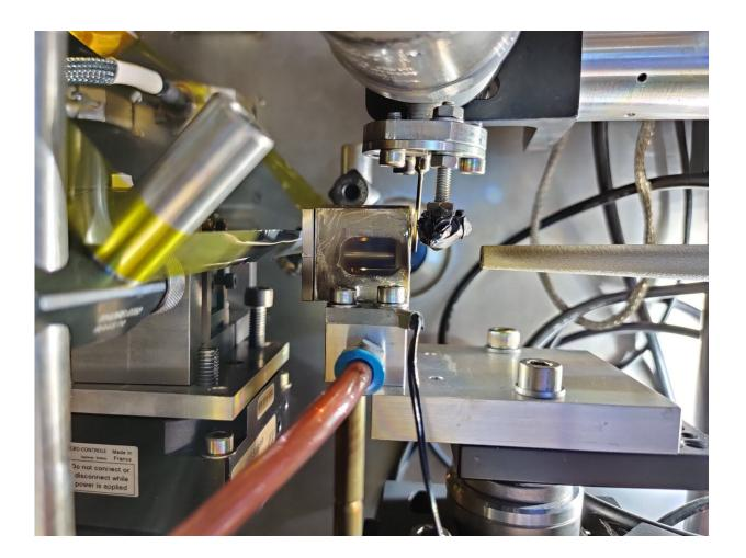
The gas cell used as a plasma source. The laser arrives from the right of these images through the metal cone and enters the little cube, which is filled with gas. The laser ionises the gas and turns it into a plasma and creates the accelerator. Credit: Rob Shalloo
