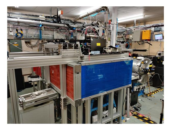
This photo shows you the outside of the vacuum chamber which is completely surrounded by painted lead bricks. The lead is for radiation protection and the metal frame allows the lead walls to be rolled in and out of the way to allow access to the chamber. They're painted because lead is highly toxic and so painting them prevents them generating harmful lead dust. Credit: Rob Shalloo
