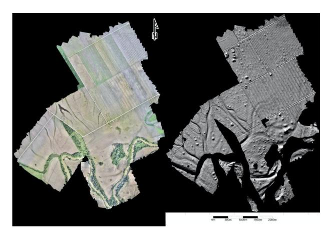
The view of fields around the Maya site of Saturday Creek, Belize. The image on left stitched together thousands of photographs into a single 3D surface. The image on the right used virtual illumination to highlight small changes in elevation to identify ancient house mounds. Credit: Models created by Mark Willis, used with permission of Eleanor Harrison-Buck, <u>CC BY-ND</u>
