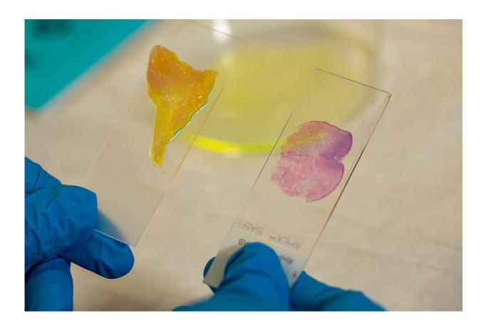
A new microscope called DeepDOF uses artificial intelligence to quickly and inexpensively image all of the cells in large tissue sections (left) at high resolution with minimal preparation, eliminating the costly and time-consuming process of mounting thin tissue slices on slides (right). Credit: Brandon Martin/Rice University
