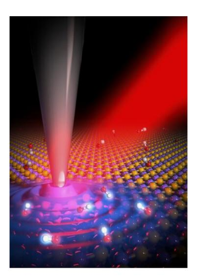
llustration of nanoimaging of molecule vibrations coupled to phonon polaritons (blue wave) in a thin boron nitride layer Credit: Scixel.
