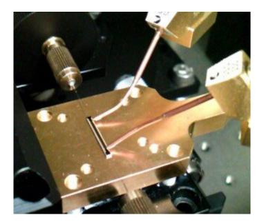
The silicon-polymer hybrid modulator seen here as a thin, black strip was developed by researchers in Japan and can transmit data at 200 Gbit/s at temperatures up to 110 °C. Modulators able to operate quickly at such high temperatures could reduce cooling demands in datacenters and unlock applications in harsh, poorly controlled environments such as cars, airplanes, and rooftops. Credit: Shiyoshi Yokoyama, Kyushu University
