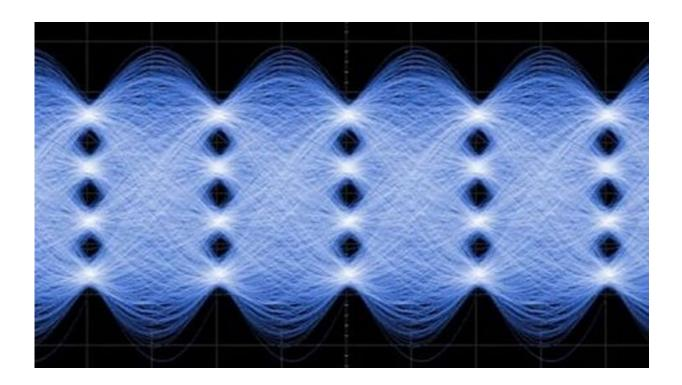
Waveforms of data transmitted at 200 Gbit/s using a hybrid-polymer modulator capable of operating at temperatures up to 110 °C. The signals can take one of four different levels that correspond to two bits each, resulting in three holes in the overlapping signals. Credit: Kyushu University
