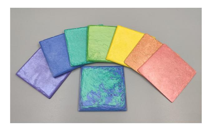
Based on different commercially available raw materials (e.g., TiO2-mica, Fe2O3-mica), a variety of all-natural bioinspired structural materials with different colors can be fabricated. Credit: GUAN Qingfang
