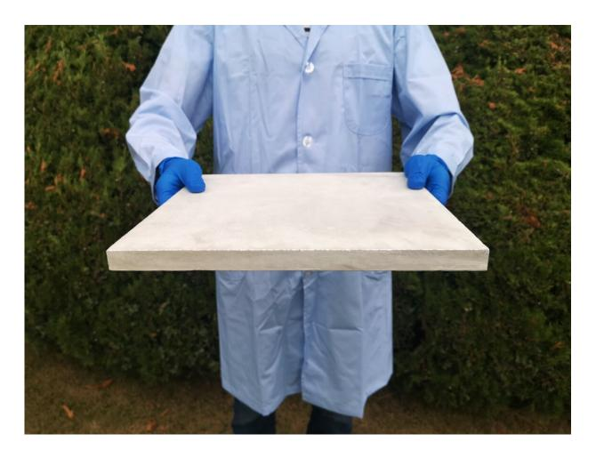
Because the proposed manufacture method, directional deforming assembly, is effective and scalable, mass production of all-natural bioinspired structural material can be achieved. Credit: GUAN Qingfang
