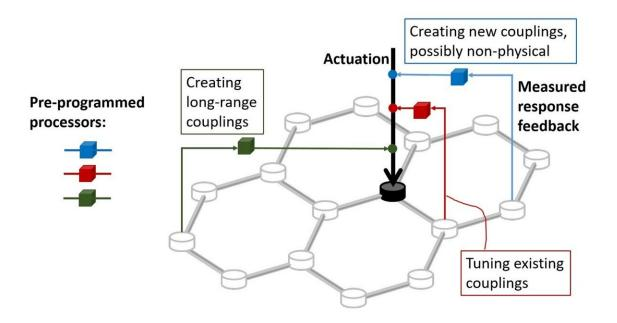
An active feedback controlled metamaterial. Whereas usually couplings between metamaterial elements are fixed, incorporating pre-programmed controllers can enable non-Newtonian mechanical interactions. Credit: Lea Sirota
