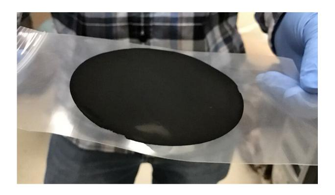
A wafer-scale composite membrane made of vertically aligned, single-walled carbon nanotubes embedded in a parylene-N polymer matrix. Credit: Lawrence Livermore National Laboratory
