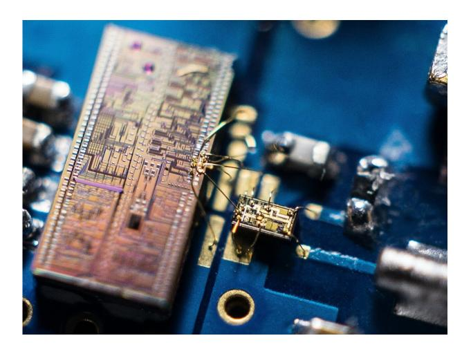
The integrated detector combines a silicon photonic chip with a silicon microelectronics chip, yielding advanced speed in detecting quantum light. Credit: University of Bristol
