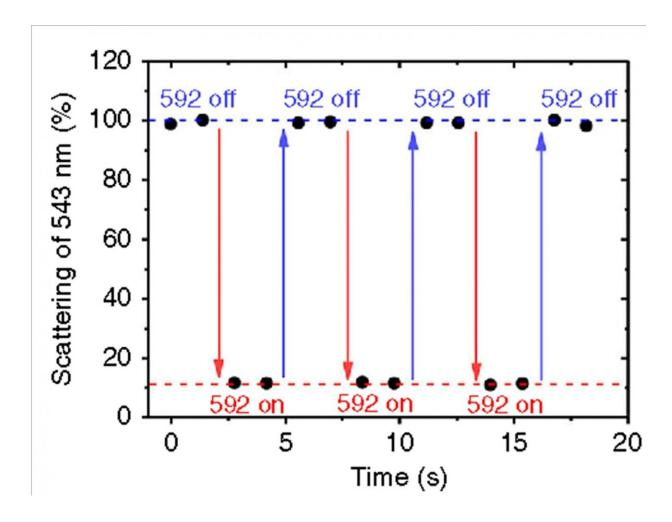
Demonstration of optical switch by controlled light (wavelength of 592 nm). The intensity of the signal light (543 nm) is switched by turning the controlled light ON or OFF. Credit: Osaka University
