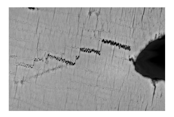
In nacre, crack propagation direction is both perpendicular (mode I) and parallel (mode II) to the tensile force. Researchers discovered that the crack-jumps (mode II) are related to the crystal orientation of the aragonite tablets. Credit: Massachusetts Institute of Technology
