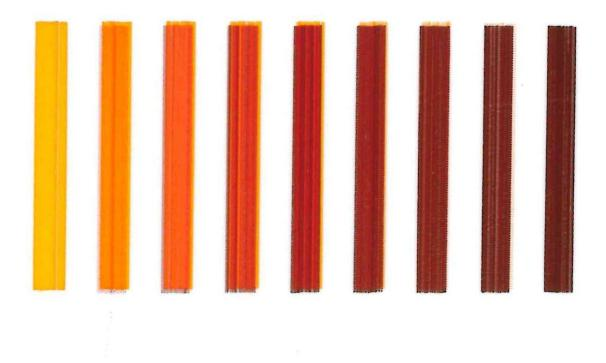
Nine samples with mixtures from CsPbBr2I (ink 1, left) to pure CsPbI3. Credit: H. Näsström/HZB
