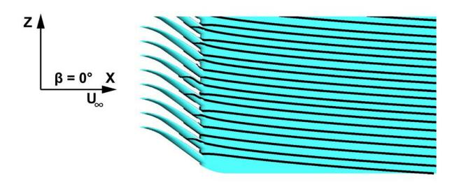
His team was surprised that instead of producing vortices, the finlets act as thin guide vanes due to their special 3-D curvature. The regular array of such finlets over the wing span therefore turns the flow direction near the wall in a smooth and coherent manner.
