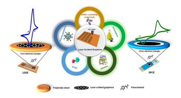
Sensing platforms using laser-derived graphene electrodes (LSGEs) exhibit higher electrochemical performances than conventional systems using carbon electrodes (SPCE) for the detection of sulfur-containing compounds, drugs, antioxidants, vitamins, catecholamines and their precursor, L-Dopa. Credit: KAUST
