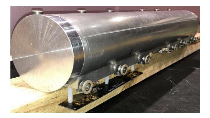
Fully assembled trolley system with wheels for riding on rails and the new external barcode reader for an exact position measurement. The 50 cm long cylindrical shell encloses the 17 NMR probes and custom-built readout and
