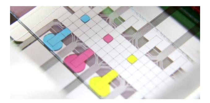
A microfluidic chip with individual droplets shown in different colors. Each droplet contains material from single cells and delivers it for single cell omics analyses. Credit: Wheeler lab
