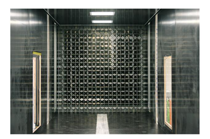
The active grid in the wind tunnel can stir up air flows to generate realistic storm turbulence. Credit: University of Oldenburg/Mohssen Assanimoghaddam
