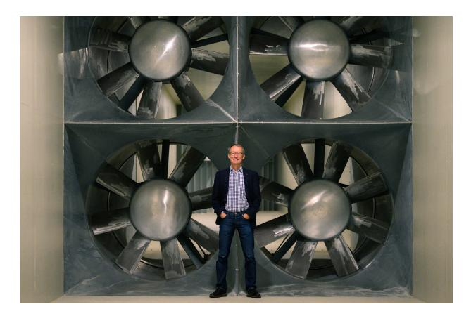
Joachim Peinke in front of the four fans of the wind tunnel. The turbines can generate wind speeds of up to 150 kilometers per hour. Credit: University of Oldenburg/Mohssen Assanimoghaddam
