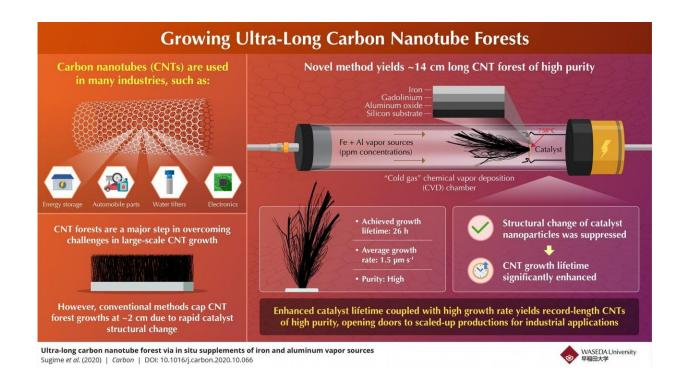
Scientists from Japan have proposed a way to ensure longer catalyst lifetime and higher growth rate, creating a CNT forest that is a record seven times longer than any existing CNT array. Credit: Waseda University
