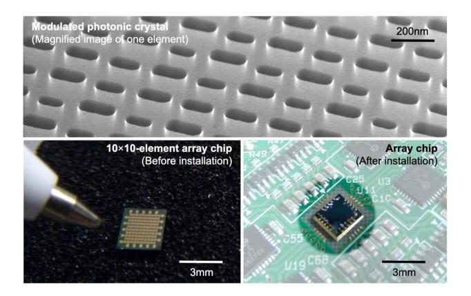
A seemingly random line of photonic crystals allows for laser beams to be emitted in various angles, allowing for more versatile and compact LiDAR technology Credit: Kyoto University/Noda Lab
