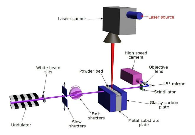
Schematic of operando synchrotron x-ray experiment on laser powder bed fusion (LPBF), with x-ray optics to control the beam, sample holder with glassy carbon plates to contain powder, scintillator to convert x-rays to light, high-speed camera to capture movies and high-power laser with scan head to deliver a laser beam to melt the surface of the sample. Credit: Carnegie Mellon University College of Engineering
