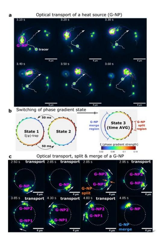
a, Multiple gold NPs (spheres of 200 nm radius) are confined by a ring-shaped laser trap (wavelength of 532 nm) and optically transported around it. These NPs rapidly assemble into a stable group of hot particles creating a confined heat source (G-NP) of temperature ~500 K. Free (not trapped) gold NPs acting as
