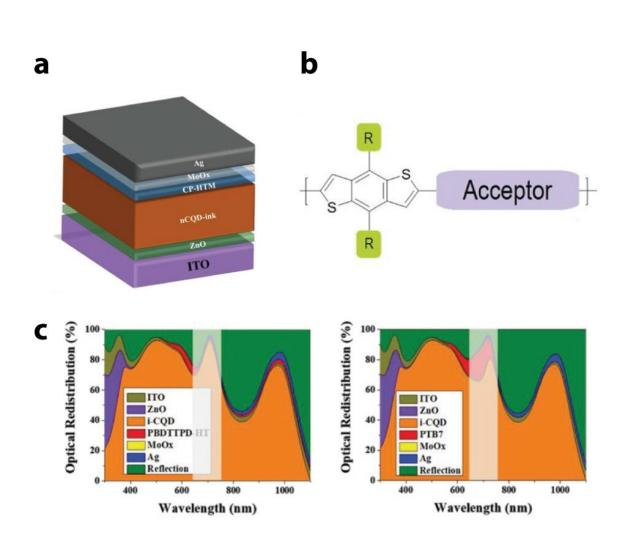
Figure 1. Shown above is the structure of CQDSC and the optical redistribution profiles of devices by TMF optical simulation. Credit: Professor Sung-Yeon Jang, UNIST
