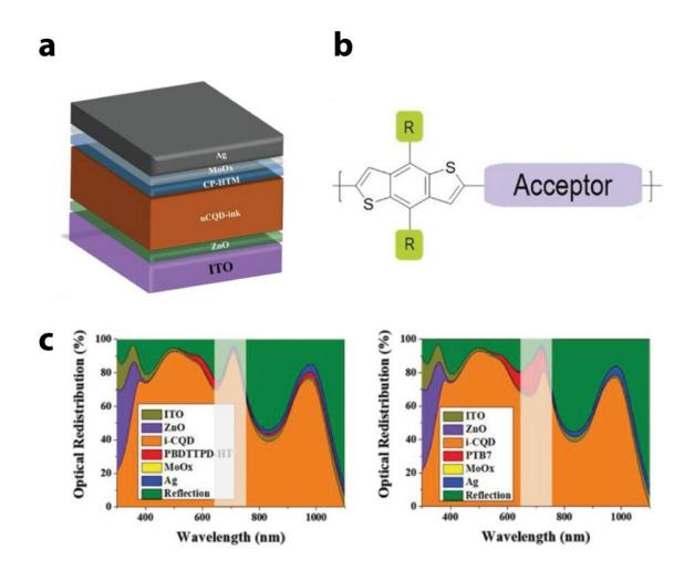
Figure 1. Shown above is the structure of CQDSC and the optical redistribution profiles of devices by TMF optical simulation. Credit: Professor Sung-Yeon Jang, UNIST
