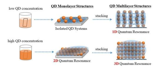
Low quantum dot concentrations during superlattice fabrication suppresses quantum resonance between dots in the same layer, while high concentrations activates it. Credit: DaeGwi Kim, Osaka City University
