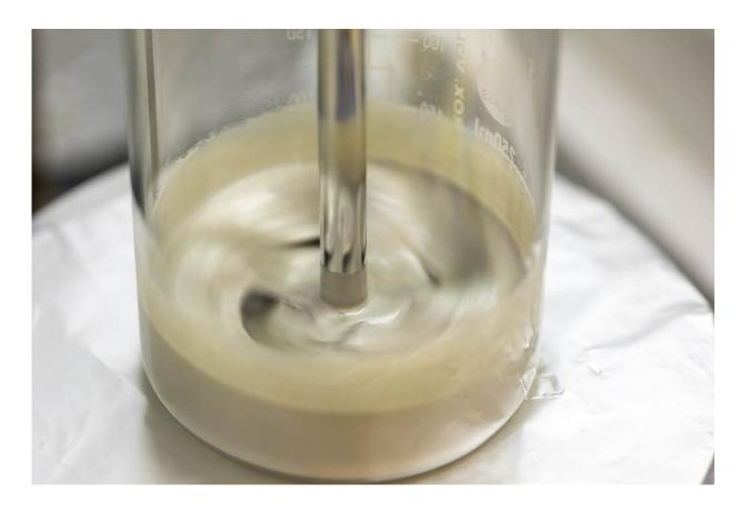
KAUST researchers developed this conductive ink by dispersing silver nanowires in a polymer solution. Credit: KAUST
