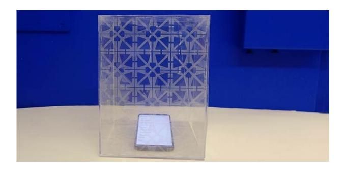
The researchers observed a significant reduction in the signal strength from a cell phone inside a box covered with their inkjet-printed electromagnetic-wave-blocking nanowire-polymer conducting sheet. Credit: KAUST
